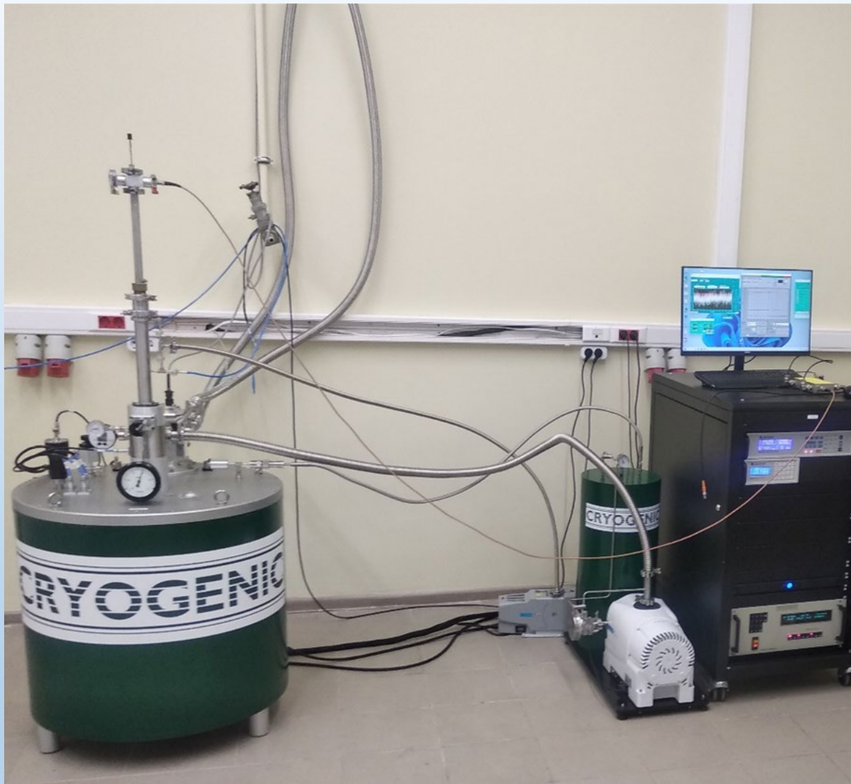
Cryogenic High Homogeneity Cryogen Free Measurement System (CFMS) 12 T , VTI 1.6 – 400 K + Digital NMR spectrometer
