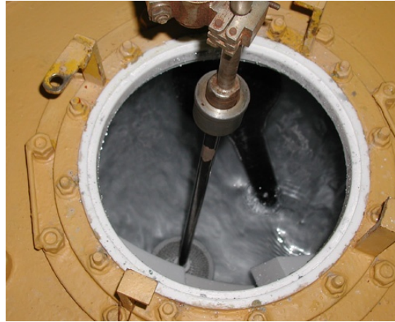
Liquid metallic Ga in the window of chemical reactor of SAGE experiment
