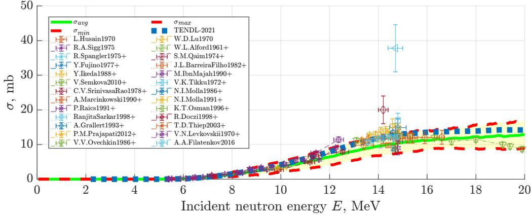
Figure 2. Formation cross section of isomeric (m) state in the  $^{90}\text{Zr}(n,p)^{90m}\text{Y}$  reaction as a function of incident neutron energy.
