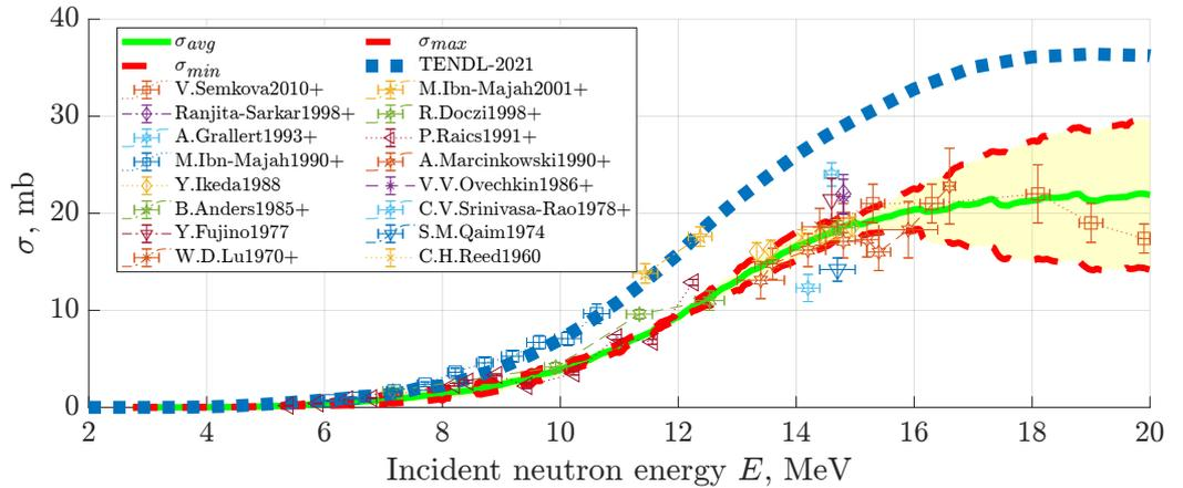
Figure 1. Formation cross section of isomeric (m) state in the  $^{91}\text{Zr}(n, p)^{91\text{m}}\text{Y}$  reaction as a function of incident neutron energy.
