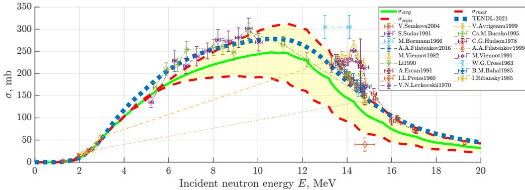
Figure 3. Formation cross section of isomeric (m) state in the  $^{58}\text{Ni}(n,p)^{58m}\text{Co}$  reaction as a function of incident neutron energy.
