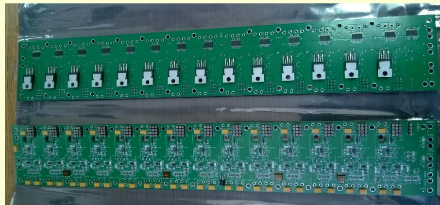
Slow control integrated to LVDB board
