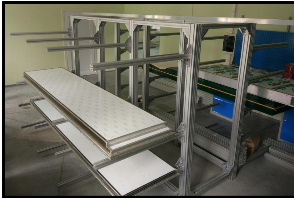
1 stand = 6 modules = 60 detectors (120 preamps + 40 TDC)
