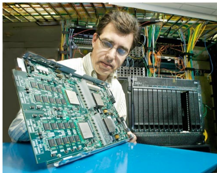
blade11bc4 @IBM, Böblingen: 2 Cell Broadband Engines, 256 kB LS, 2.4 GHz
