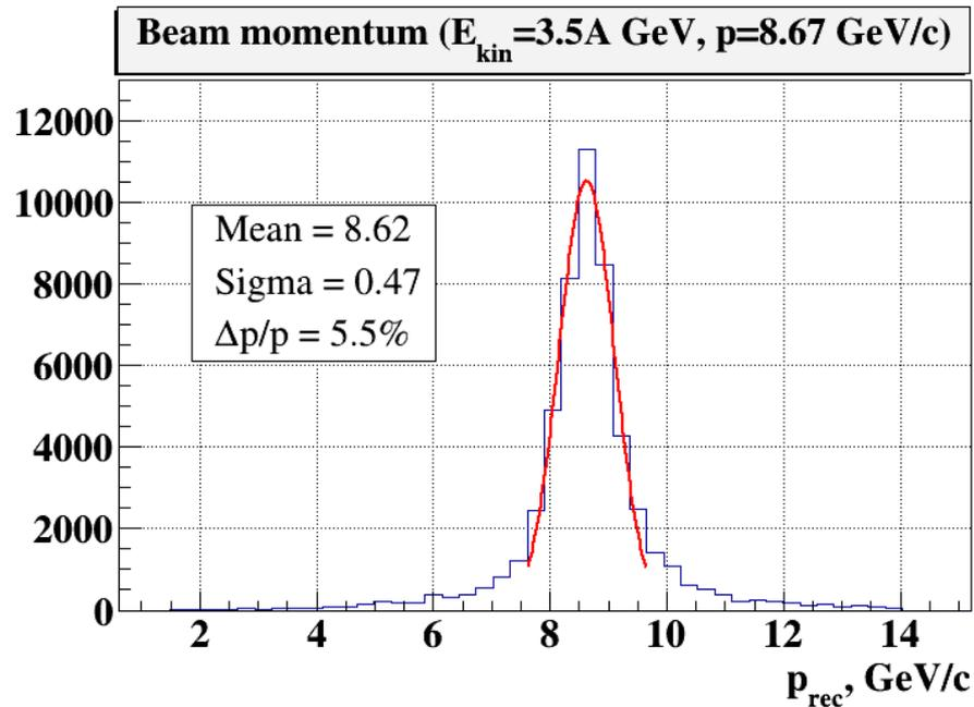
Carbon beam, gas in GEM: Ar+CO<sub>2</sub>
