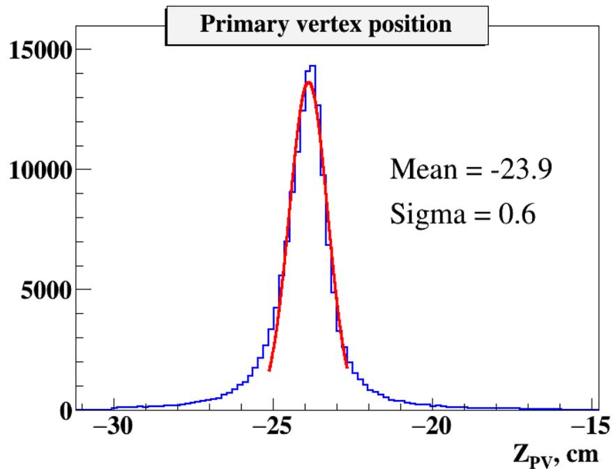
Primary Vertex with Si detector & Pile-up suppression.
