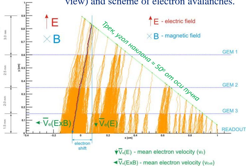
Profile of electron avalanche at the readout-plane (cluster).
