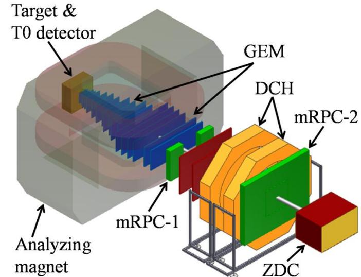
**BM@N advantage:** large aperture magnet (~1 m gap between poles)
