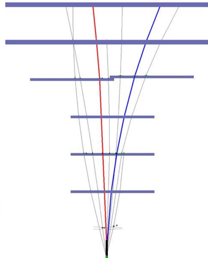
***Event Display:*** Example of the  $\Lambda$  decay reconstruction in the tracker (GEM + Si) in C+C interaction.
