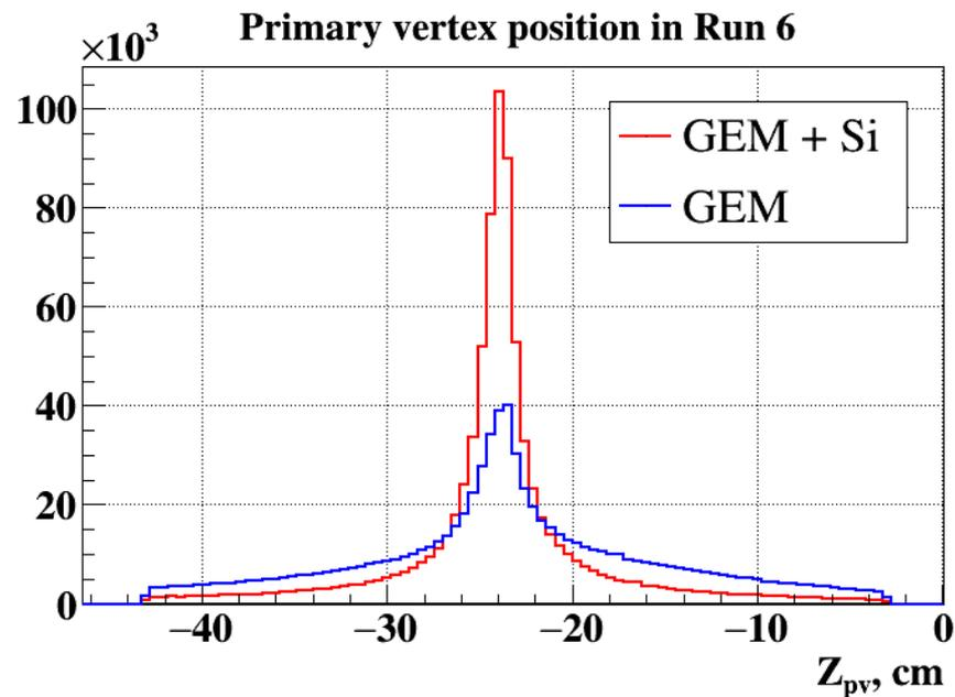
Primary Vertex with Si detector vs without Si detector.
