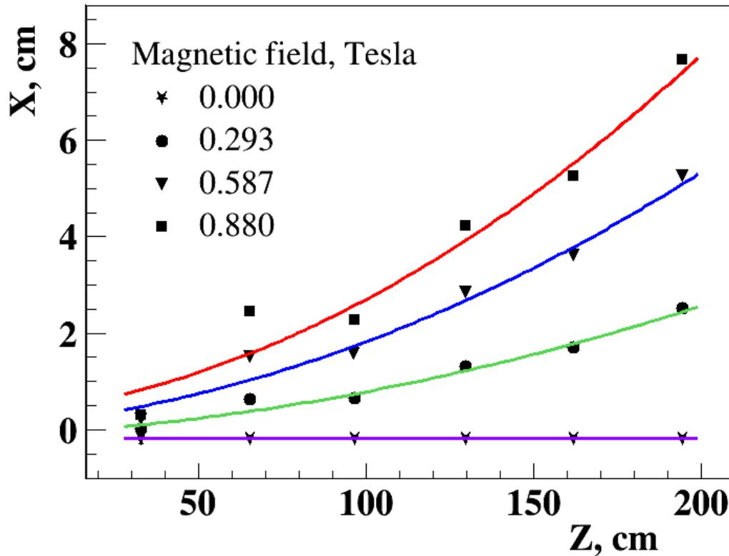
Averaged positions of deuteron beam with  $E_{kin} = 4A$  GeV reconstructed in 6 GEM planes at different values of magnetic field
