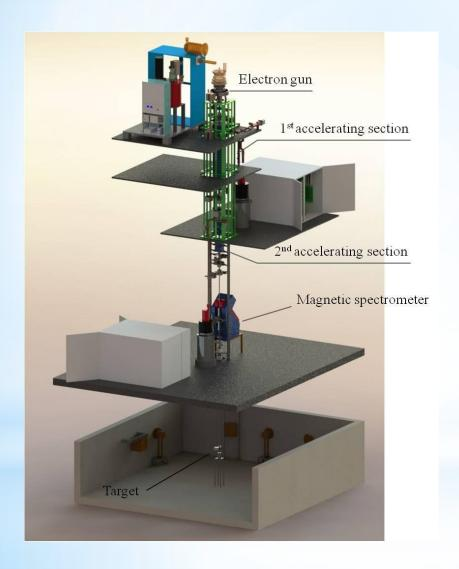
The main part of the IREN facility is a linear electron accelerator. The bunched electron beam generates bremstruhlung in the tungsten target and it produces the neutron pulses via  $(\gamma,n)$ -reaction in the same target.
