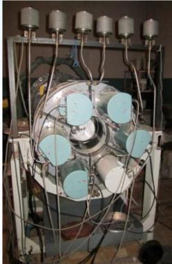
Detector contains 6 sections forming together the cylinder with the channel along the beam direction. neutron Diameter of the channel is 300 mm, external diameter of the detector is 730 mm, length 600 mm. Total volume of liquid scintillator is 250 liters. There are photomultipliers in both ends of each section. The signals from two photomultipliers of each section are summarized on output load resistor.
