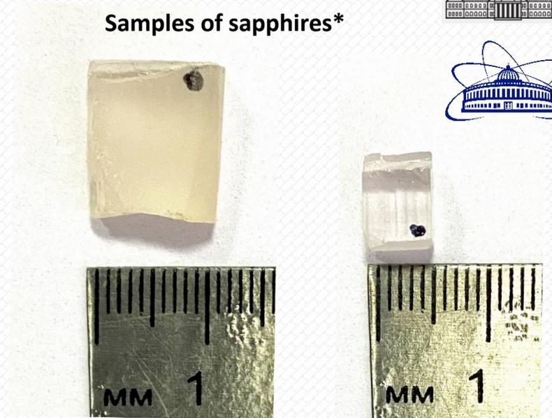
\*Transparent wedge-shaped samples of crystalline alumina (sapphire) produced by the Verneil method.
