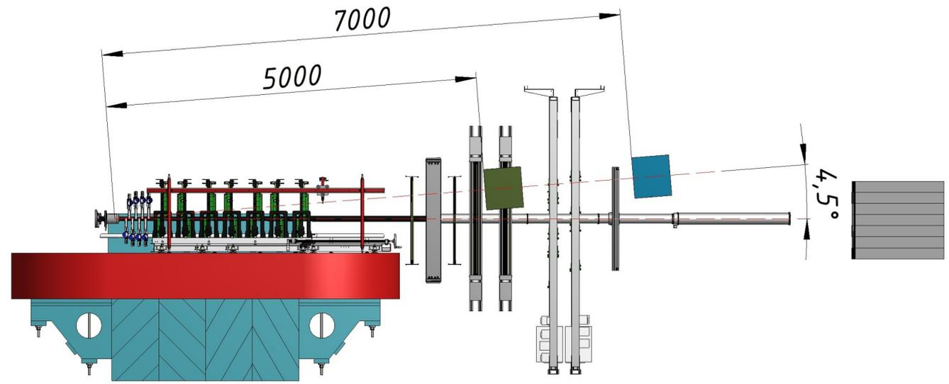
Rotation in Y-Z plane will help to minimize of material budget on the way of neutrons from the target to the HGND
