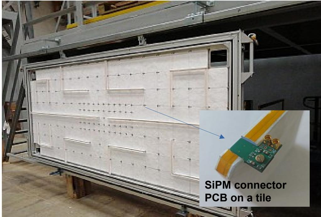
ScWall mounted on the frame during Run8 run
