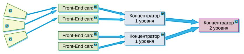
• It is necessary to have a mapping of the data collection system that establishes the correspondence of the channel addresses at the DAQ outputs with the devices from which this signal came
