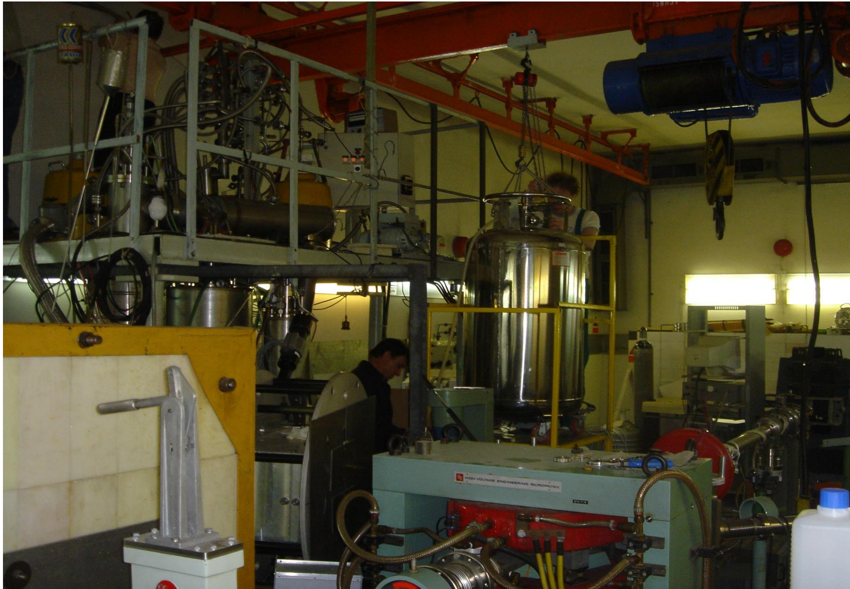
Target with a frozen nuclear polarization for experiments at low energies in Prague. NIM A 345, (1994) 421-428.
