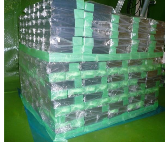
Lead after acid cleaning
