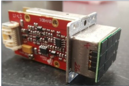
Single SiPM array with 2 preamps
