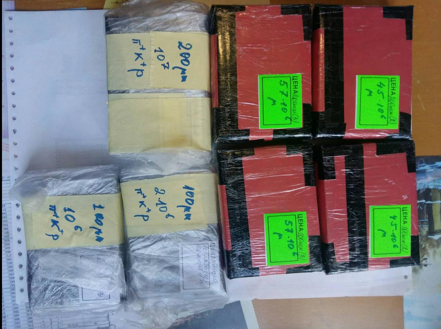
Three stacks of 10 layers with an emulsion thickness  $1000 \mu\text{m}$  and 3 of 10 layers with a thickness of  $200 \mu\text{m}$  are irradiated perpendicular to the beam. Nearby monitor is  $8 \times 8 \text{ cm}^2$ . The fluences are  $9.3 \times 10^6$ ,  $45 \times 10^6$ , and  $57 \times 10^6$ . The average energy of muons is 2.5 GeV on average.
