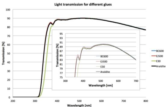
The various glues on the epoxy base (EJ-500, Aqua E-300, BC-600 and Araldite Crystal) are often used as a filler in the groove of tiles. Transmittances (T) of their unirradiated samples  $T > 90\%$  for  $\lambda > 400\text{nm}$  are showed on the left figure)
