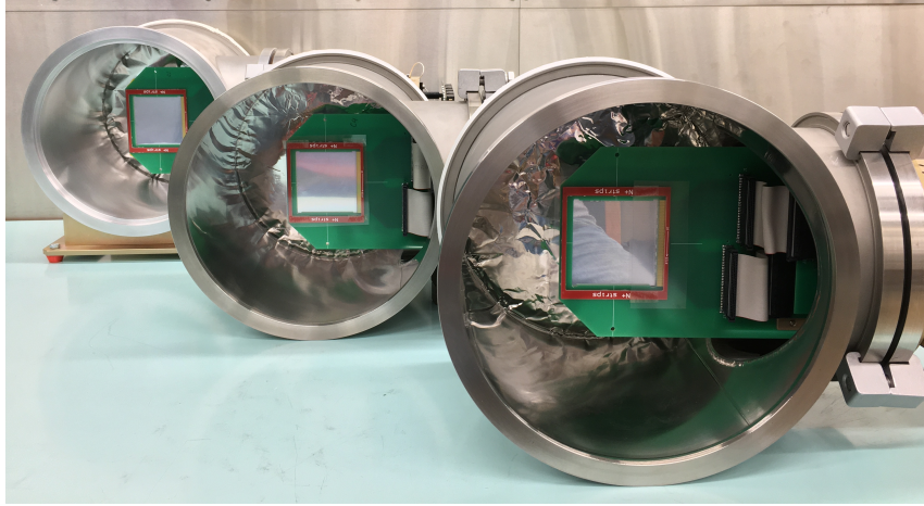
Figure 15: Three stations SiBT1, SiBT2, SiBT3 with detectors and FEE electronics, view along the beam ( p^+ side of the strips).
