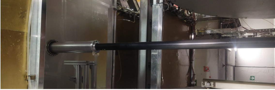
Figure 6: Carbon beam pipe connected by a flange to aluminum beam pipe in the BM@N setup.
