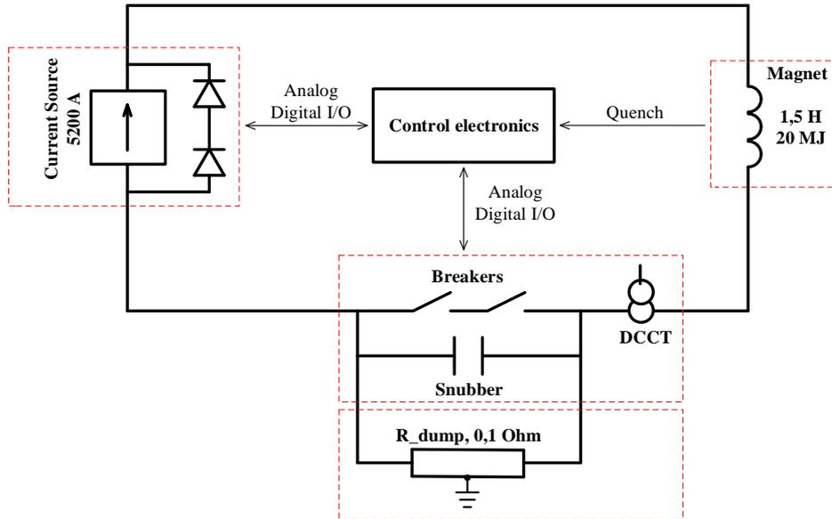
The quench protection system (QPS) is designed to limit the peak temperature on the coil windings to 80 K and the peak voltage to ground to 500 V during any normally protected quench. The system relies on the monitoring of the resistive voltages associated to the normal zone spread and quench development via voltage taps installed on the coil modules as well as on the joints and bus bars.
