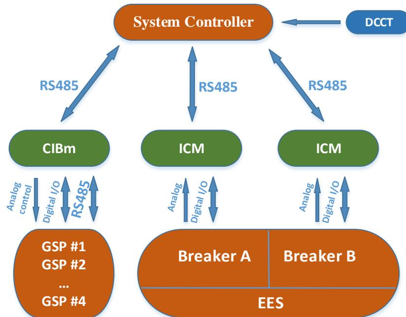
Energy extraction system for redundancy consists of two breakers, therefore, we need two undependable ICM modules to follow the redundancy principle of two breakers control. First ICM controls Breaker A, and second – Breaker B. Digitizing of analog signals is shared between to ICM modules.
