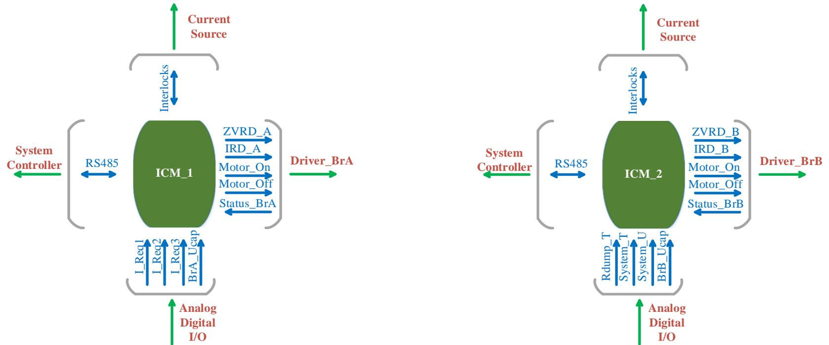
ICM#1 controls Breaker A by four digital signals: ZVRD\_A (zero voltage release device, BrA), IRD\_A (independent release device, BrA), Motor\_ON\_A, Motor\_OFF\_A (motor drives). Furthermore, ICM#1 receives statuses of Breaker A, digitizes current sharing analog signals and monitors the voltage of the buffer capacitor on the Breaker A driver board - U\_cap\_A.
