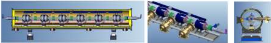
The collider Higgs mode for 30 MW SR power per beam will use 32 units of 11 m-long collider cryomodules will contain six 650 MHz 2-cell cavities, and therefore, a full size 650 MHz cryomodule will be developed in EDR
