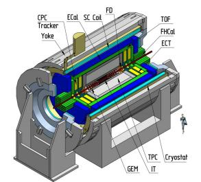
Time Projection Chamber (TPC) is a main tracking detector, overlapping pseudorapidity region  $|\eta| < 1.5$  with high particle reconstruction efficiency for  $p_T > 0.1$  GeV/c
