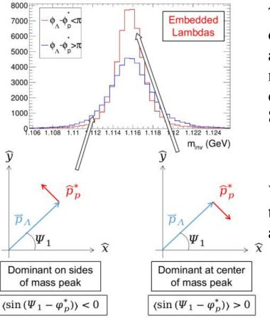
This method can deal with tracks crossing: daughter particles tracks with opposite charges are bended in the opposite directions in the magnetic field, and these tracks may cross each other -> creates 2 peaks distribution. Solution: fit Sig with 2 gausses
