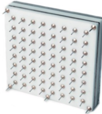
NNVT N6021 (China) 8x8 pixels with 5.9x5.9 mm
