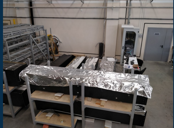
Fig. 5 Special setup for testing ECal half-sectors at JINR
