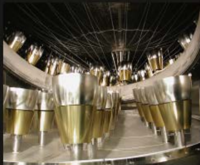
Internal view of the Borexino liquid scintillator containment liquid scintillator vessel. From the photo several parts of the detector are visible: the photomultipliers (silver-like color), the mu-metal shielding (brass-like color), the bottom of the outer nylon vessel (upper part of the photo).
