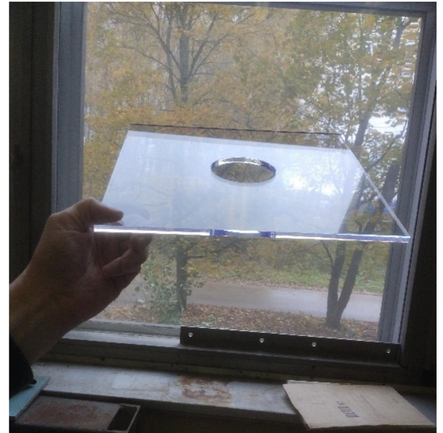
Final WLS OD plates after laser cutting and polishing
