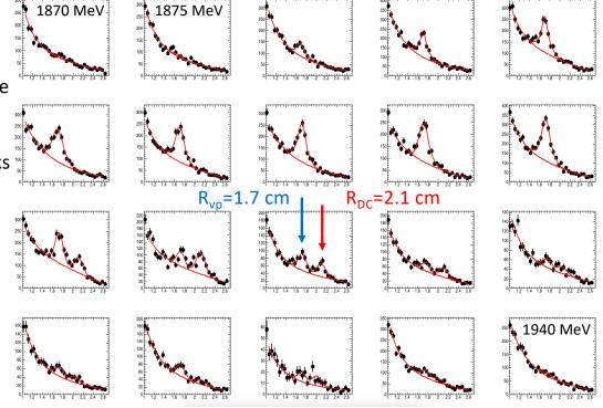
First peak – radius of the aluminum vacuum pipe  $R_{vp}$  = 1.7 cm, (0.5 mm) Second peak – inner wall of the DC carbon fiber  $R_{DC}$  = 2.1 cm (0.25mm)
