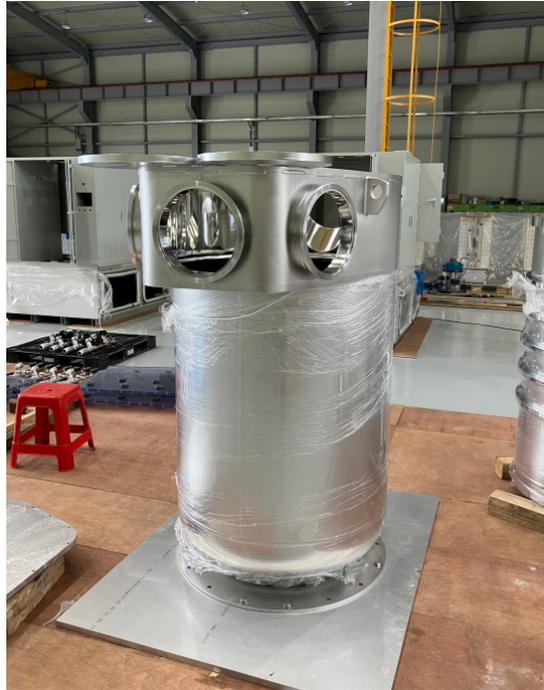
*Cryostat nearly complete, PMTs acquired*
