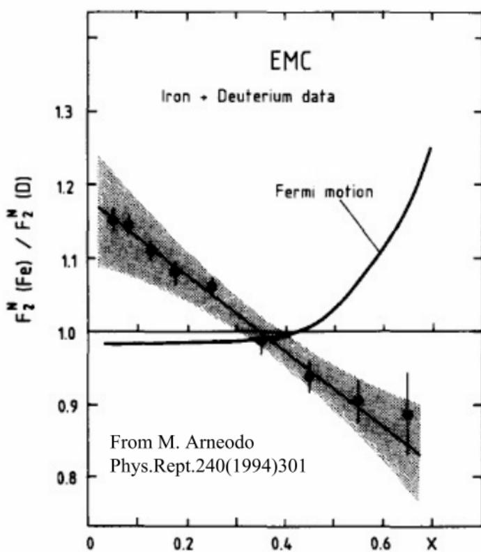
Direct measurement by [EMC Collaboration](#), 1983 indicated unexpected nuclear effects even in the DIS region. Exciting observation, although the small- $x$  part turned out to be time dependent (the effect changed sign with time).
