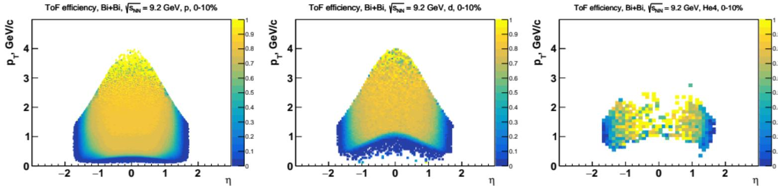
$$ToF\ efficiency = \frac{hv\_eff\_pdg\_primary\_nhits\_dca\_tof}{hv\_eff\_pdg\_primary\_nhits\_dca}$$
