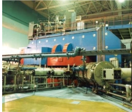
U-400M cyclotron: heavy ions 50 MeV/u (Li-Ne)
