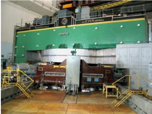
cyclotron MSC230 (since 2024): protons up to 230 MeV
