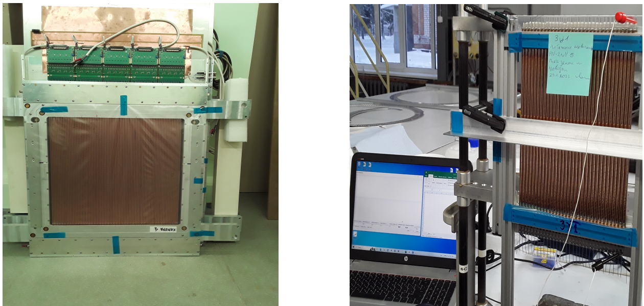
Fig.11. Left panel: existing 50 \times 50 \text{ cm}^2 straw chambers. Right panel: test of the one plane 20 \times 20 \text{ cm}^2 straw chamber for SPD test zone.
