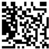
Figure 6.6 The distribution of two phases (black and white) on a square lattice in two spatial dimensions. Domain walls lie at the interface of the black and white regions.
