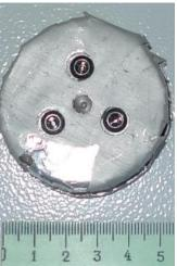
Culet size – 0.8 mm Volume – 0.02 mm<sup>3</sup> Pressure - 35 GPa Exposition time – 48 h
