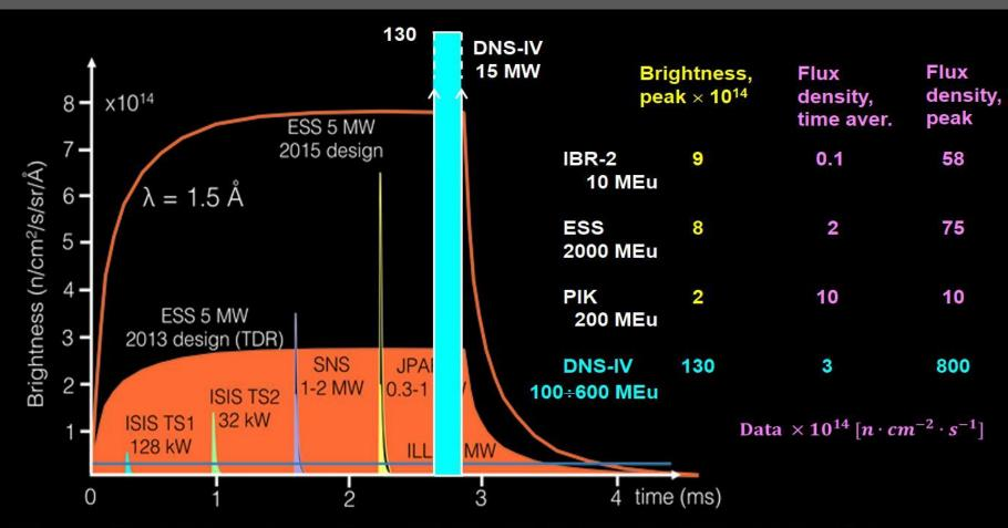
Single-pulse source brightness as a function of time at wavelenght of 1.5 A at ESS, ILL, SNS, J-PARC and ISIS Target Stations 1 and 2. In each case, the thermal moderator with the highest peak brightness shown. (Source: ESS)
