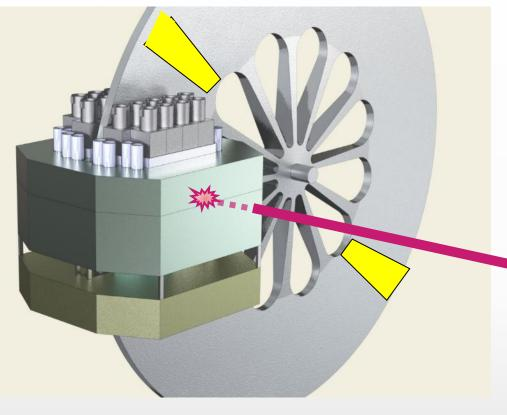
Multiplying target: Modulation of reactivity Neptunium subcritical system Long pulse ≤ 300 μs Short pulse 20 μs
