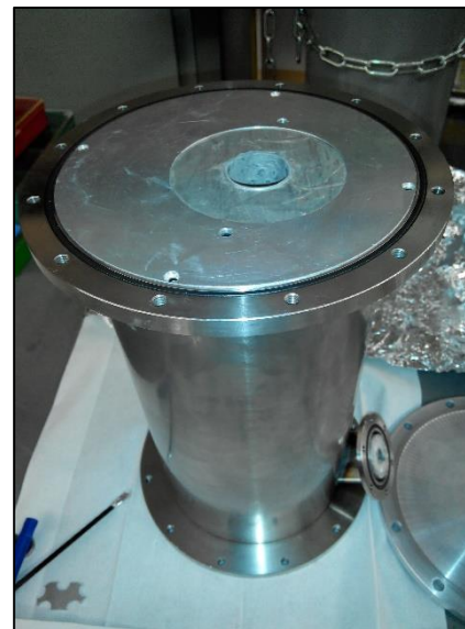
Photos of an evacuated volume of the reflector (on left) and the installation setup (on right).
