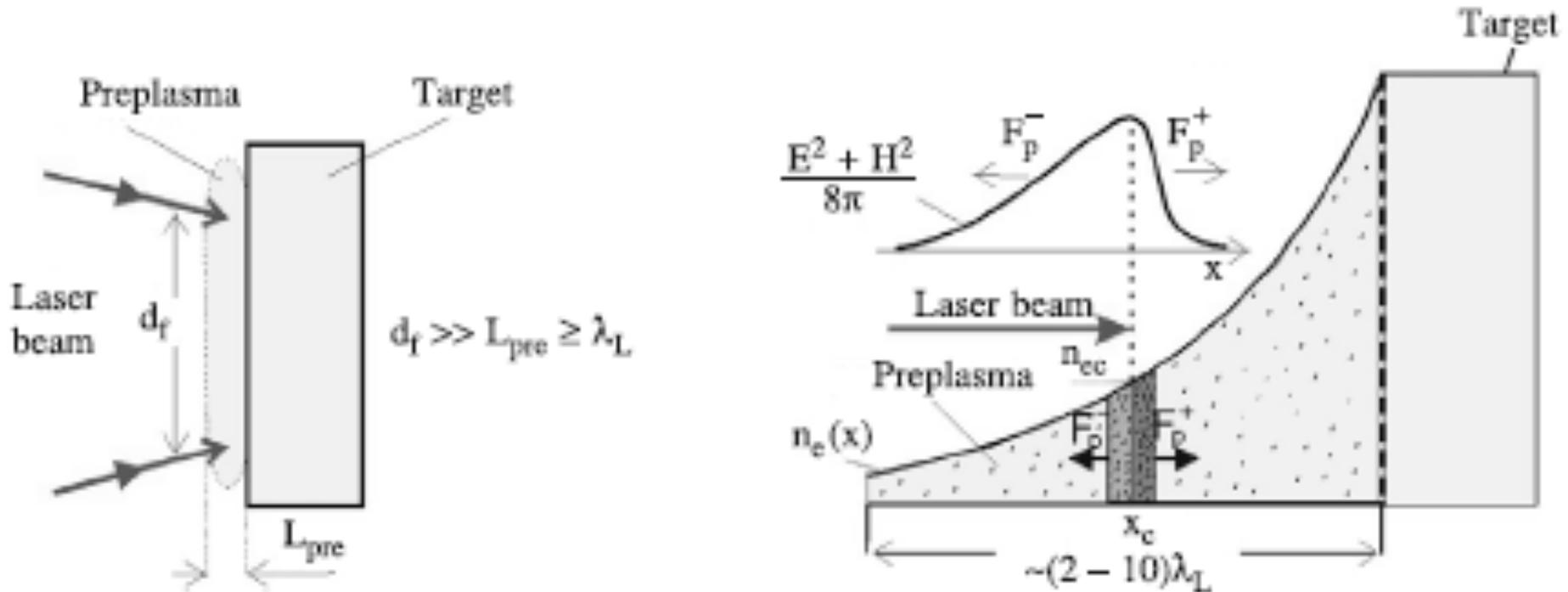
Idea of production of ion beams by S-LPA.
