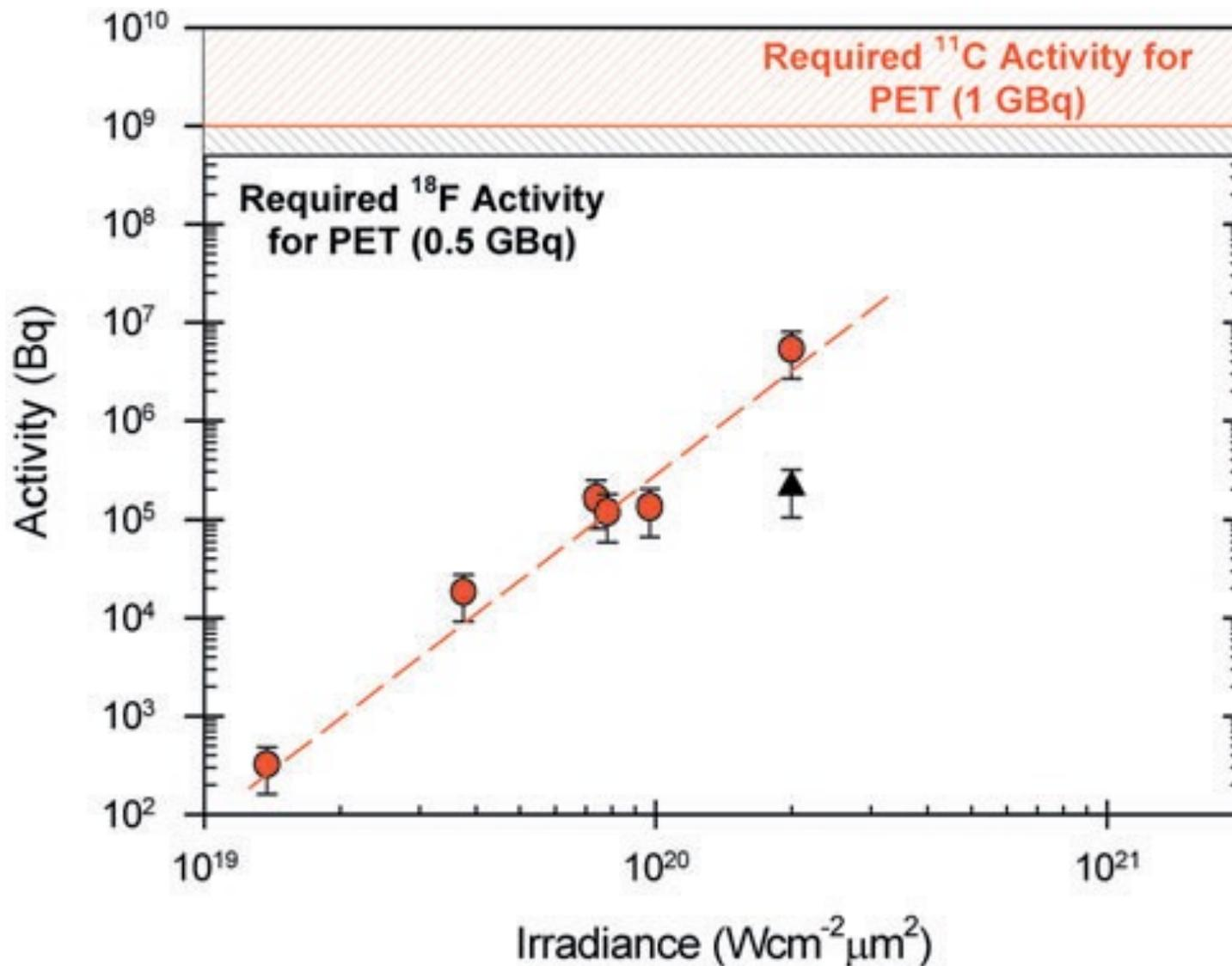
Total activity generated by a single laser shot (pulse energies from 15 to 300 J)
