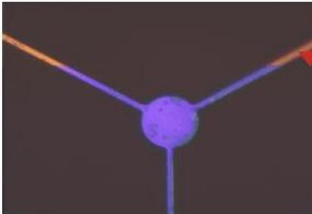
Disks: 32µm diameter, 40nm thick SiN membranes
