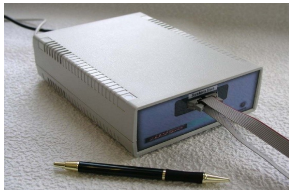
Figure 3.3.1.2: Control Units (Communication base voltage generation).
