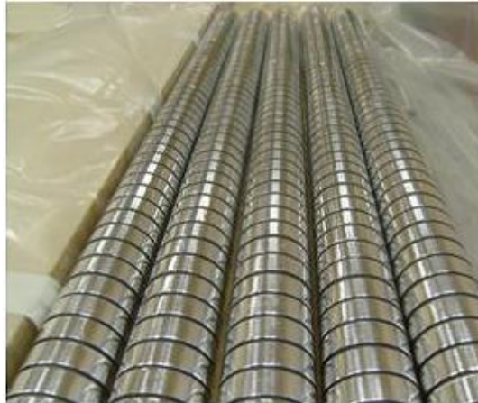
Figure 3.8: Potential degrader rods produced by industry using composite material (Kevlar + Macrolon + Al foil)
