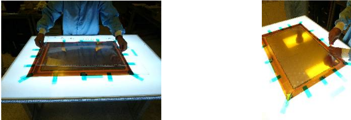
Figure 11.2: Assembly of detector based on 3 pc GEM-foils
