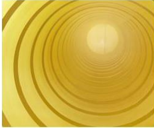
Figure 3.5: View of the 340 cm prototype vessel, produced to elaborate technology of aluminum foil strips gluing on inside wall of 600 mm diameter
