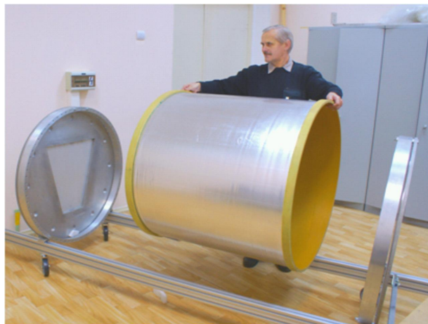
Figure 9.4: Prototyping of the TPC with Industry (Material: Kevlar laminated by Tedlar film)
