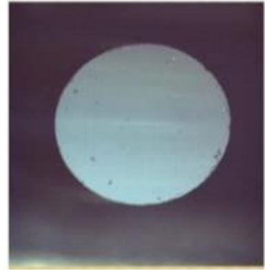
Figure 5.7: Photo of the mirror surface viewed with electron microscope after 1.5 \cdot 10^6 UV laser shots
