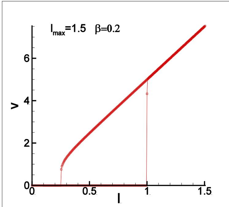
$$\begin{cases} \frac{\partial \varphi}{\partial t} = V \\ \frac{dV}{dt} = I - \sin \varphi - \beta \frac{\partial \varphi}{\partial t} \end{cases}$$
