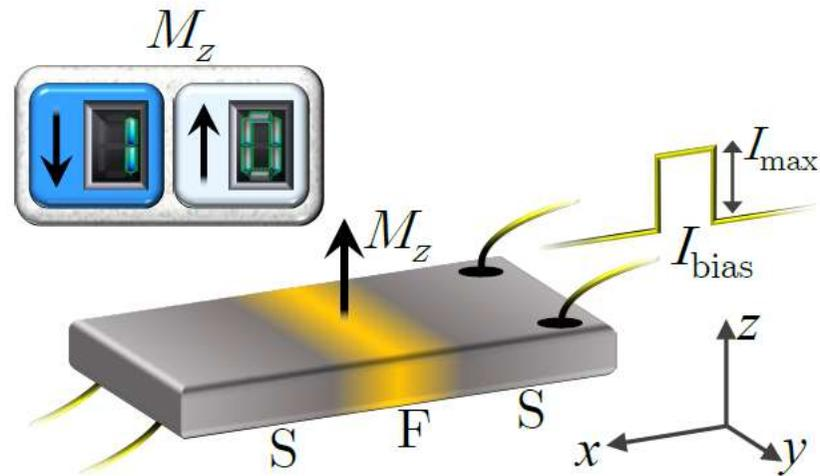
FIG. 1. S/F/S Josephson junction driven by a rectangular bias current pulses,  $I_{\text{bias}}$ , with amplitude  $I_{\text{max}}$ . The z-component of the magnetization,  $M_z$ , is the observable used to define the logic memory states 0 and 1.
