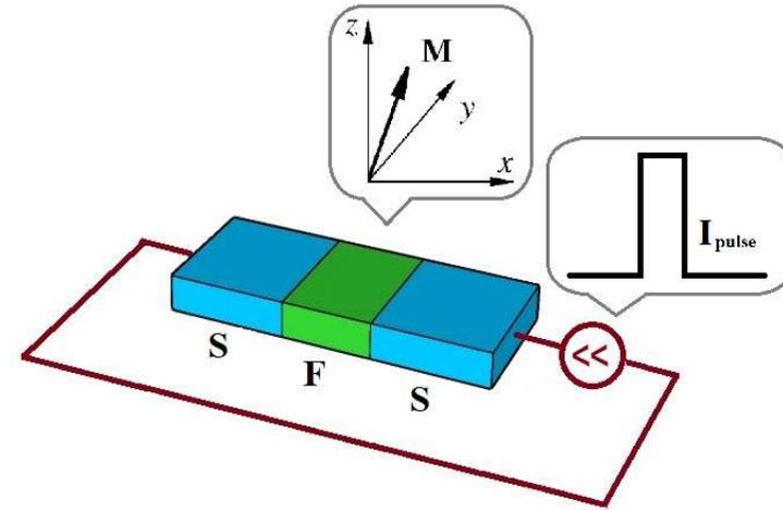
$$I_{pulse} = w \frac{d\varphi}{dt} + \sin(\varphi - r m_y)$$
