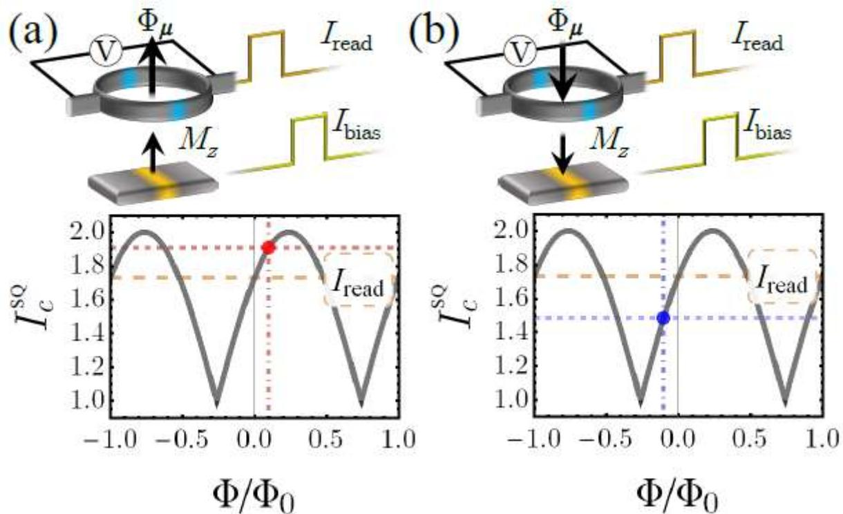
FIG. 10. SQUID-based memory readout and cartoon showing the critical current interference pattern of the SQUID, in the cases of both positive and negative orientation along the z-axis of the magnetic moment, see panel (a) and (b), respectively.
