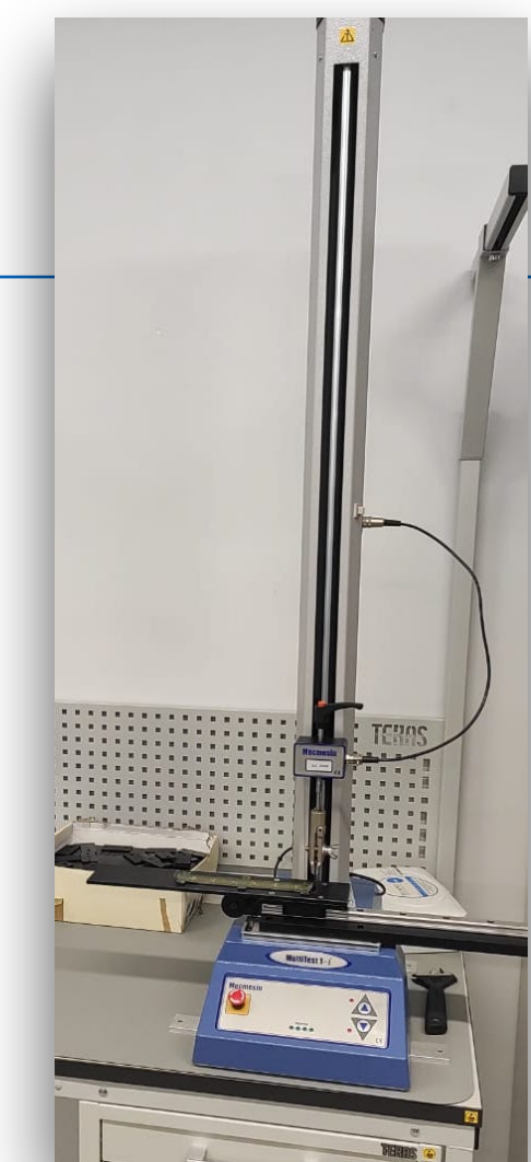
Peel test station
