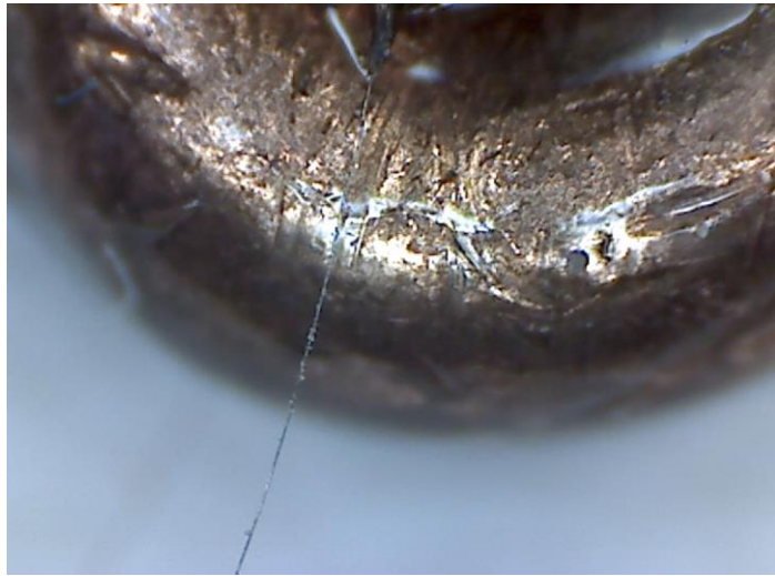
W-wire \varnothing 6 \mu\text{m} and Cu-wire \varnothing 1 mm.
