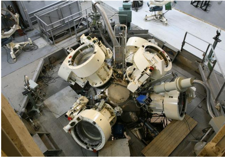
Target camera of the Iskra-5 laser system ( Institute for Experimental Physics – Sarov ).
