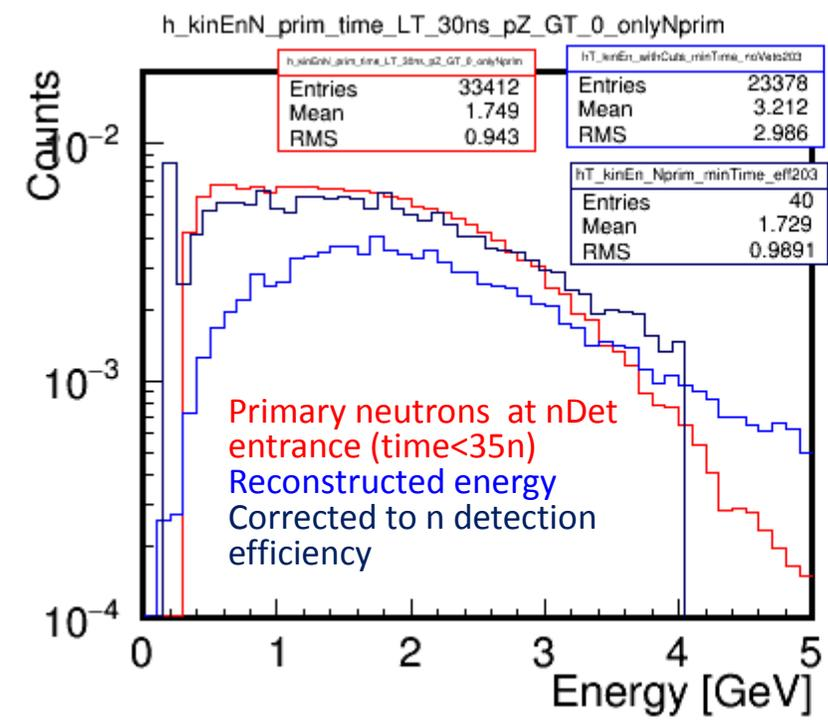
Neutron energy in events with only one primary neutron can be correctly reconstructed by determining fastest time in the HGND cells.
