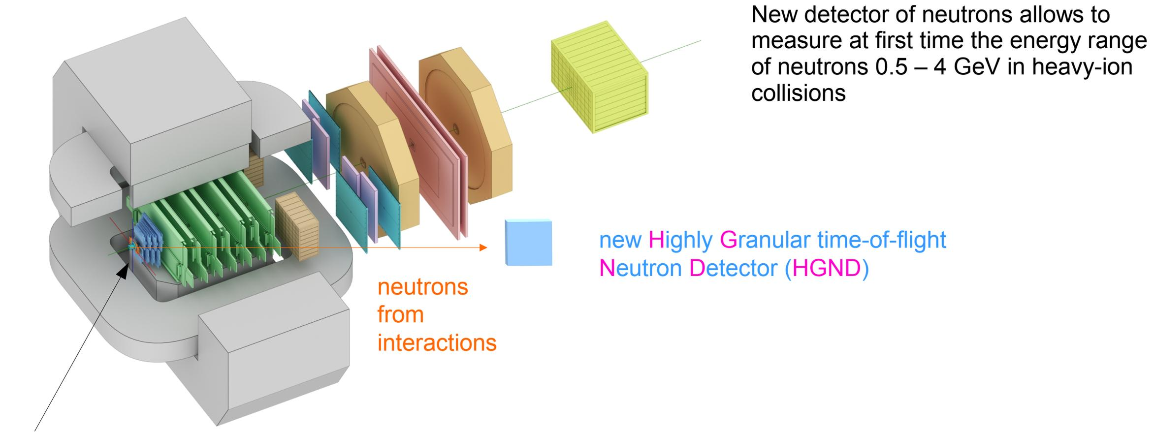
New detector of neutrons allows to measure at first time the energy range of neutrons 0.5 – 4 GeV in heavy-ion collisions
