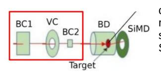
The efficiency to get a trigger signal based on multiplicities of fired channels in the BD (SiMD) detectors strig was calculated for events with reconstructed protons, deuterons and tritons using experimental event samples recorded with an independent trigger based on the SiMD(BD)detectors:
