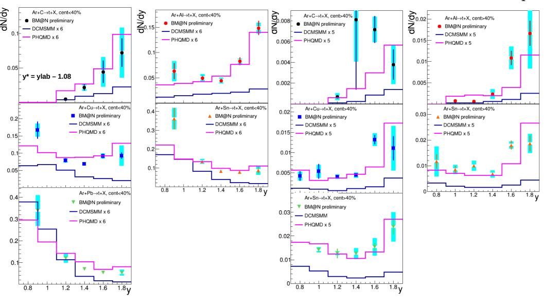
The models reasonably describe the shape of the experimental spectra, but under-predict the normalization of the data by factors of 5-6
