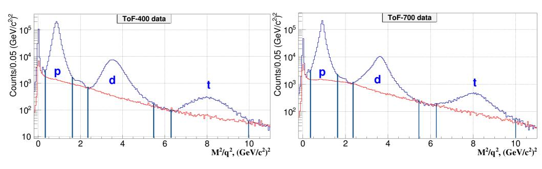
Vertical blue lines indicate the signal ranges of identified protons, deuterons, and tritons. Red lines show the background estimated from "mixed" events.
