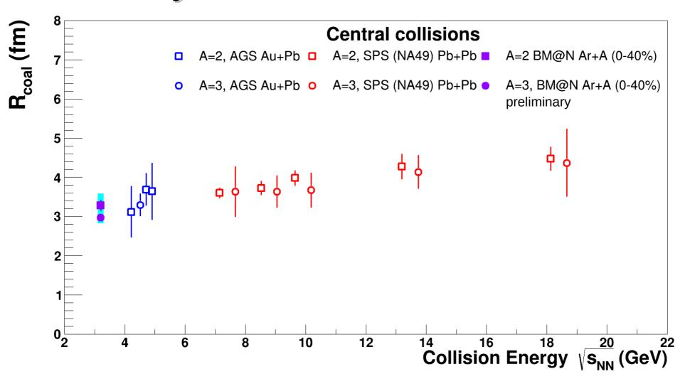
The coalescence radii calculated from B₂ and B₃ for deuterons and tritons produced in Ar+A interactions (centrality 0-40%) align with values ranging from 3 to 3.5 fm
