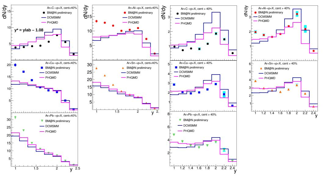
The models reasonable describes the experimental results in the forward y range. At mid-rapidity the models under-estimate the data for interactions with the targets heavier than the carbon.
