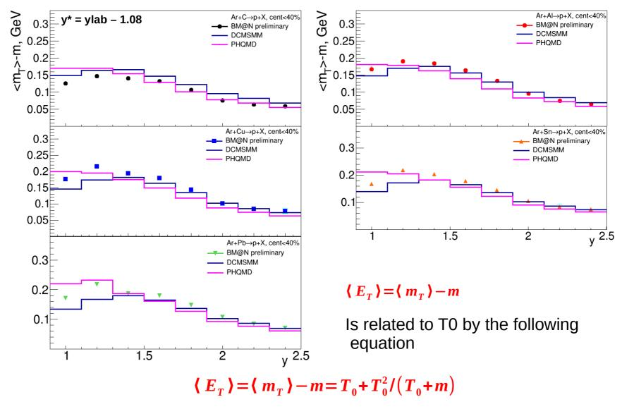
The maximal values of  $\langle E_T \rangle$  are measured at rapidity 1.0 < y < 1.3. In general, the y dependence of  $\langle E_T \rangle$  for protons is consistent with predictions of the DCM-SMM and PHQMD models.
