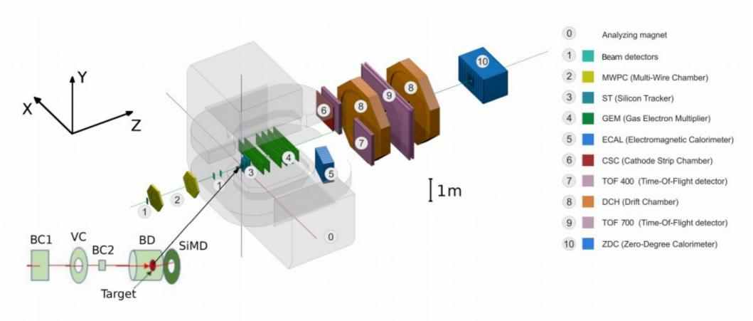
Detectors used in the analysis: Beam detectors (1), Multiplicity Detectors, ST (3), GEM (4),CSC (6), TOF 400 (7), DCH (8), TOF 700 (9)
