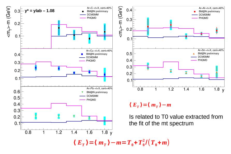
The PHQMD model reproduces the rice of the data at mid-rapidity in CM, while the DCM-SMM model predict the values which are lower than the experimental results.
