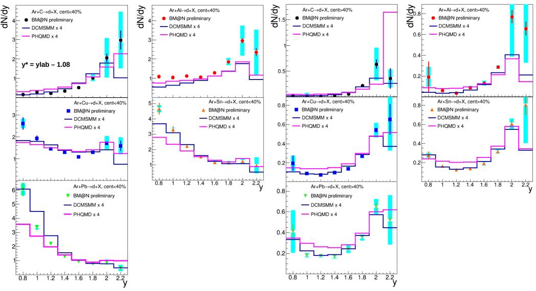
The spectra of deuterons dominate in the beam fragmentation range for Ar+C and Ar+Al interactions, whereas the spectra become more central for interactions with heavier targets. The models reasonably describe the shape of the experimental spectra, but under-predict the normalization of the data by factors of 4
