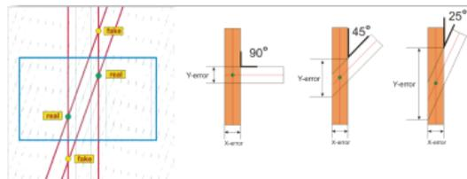
Number of "fakes" can be decreased by decreasing angle between strips in two readout planes (upper and lower layers)
