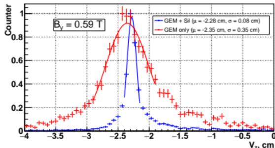
Primary vertex is reconstructed by **method of virtual planes**
