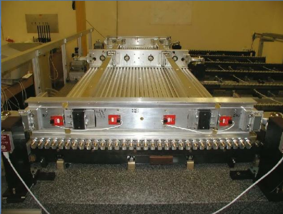
CERN ATLAS Muon Chamberon granite montage table at JINR laboratory of Nuclear Problems; new montage assembling table was done by Hi-Tech Group
