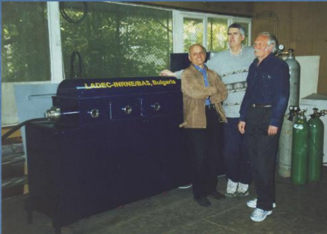
20 Joules TEA pulsed CO 2 laser as a Dubna Nuclotron ion source at LADEC test laboratory; Dr.Iv.Tsakov,Dr.D.Dimitrov, Dr.V.Monchinskii
