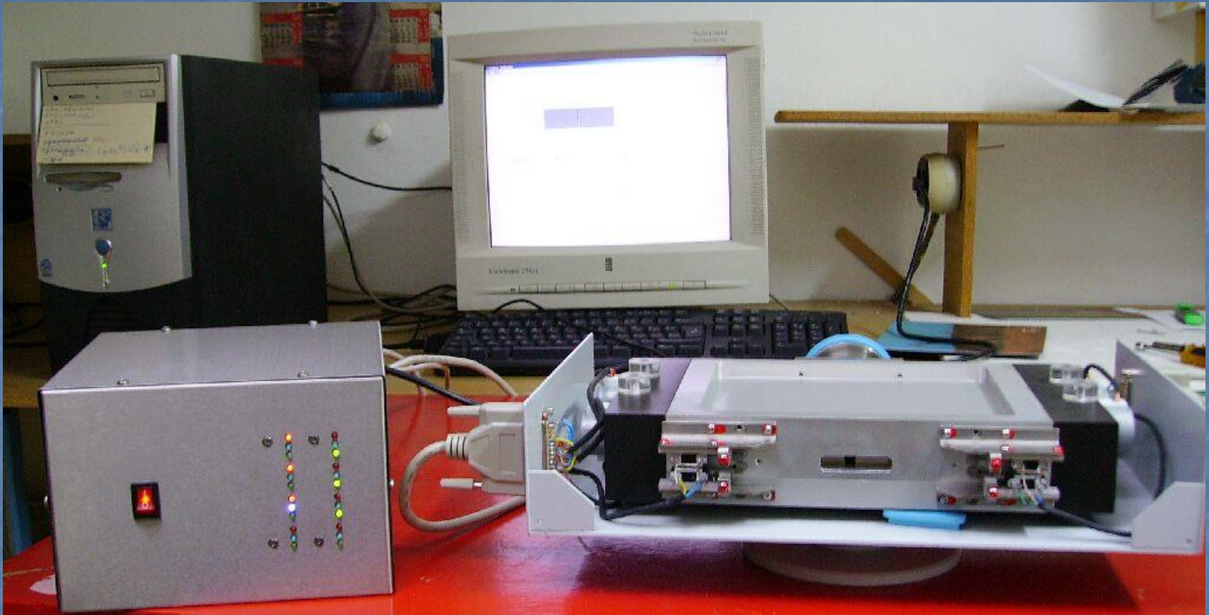
Sixth-leafs collimator for precise cancer radiotherapy at human eyes and brain for Dubna accelerator medical beams
