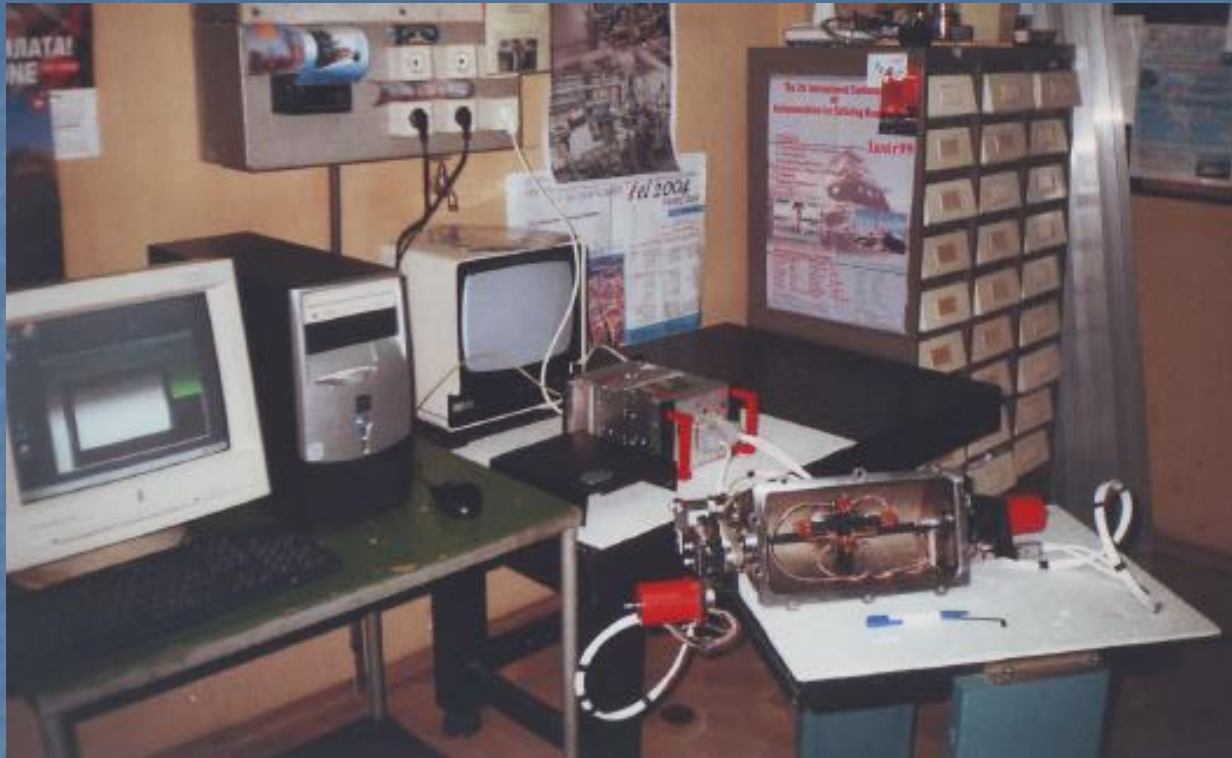
Computerized precise XY target for the Dubna Nuclotron laser ion source under laboratory test at INRNE Hi-Tech laboratory
