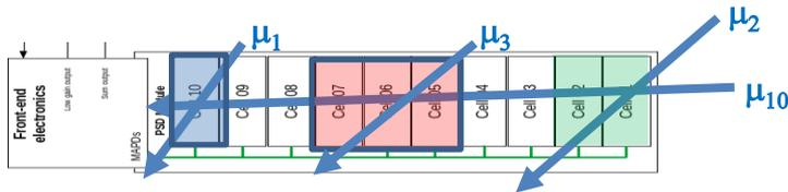
Measurement with horizontal and inclined tracks
