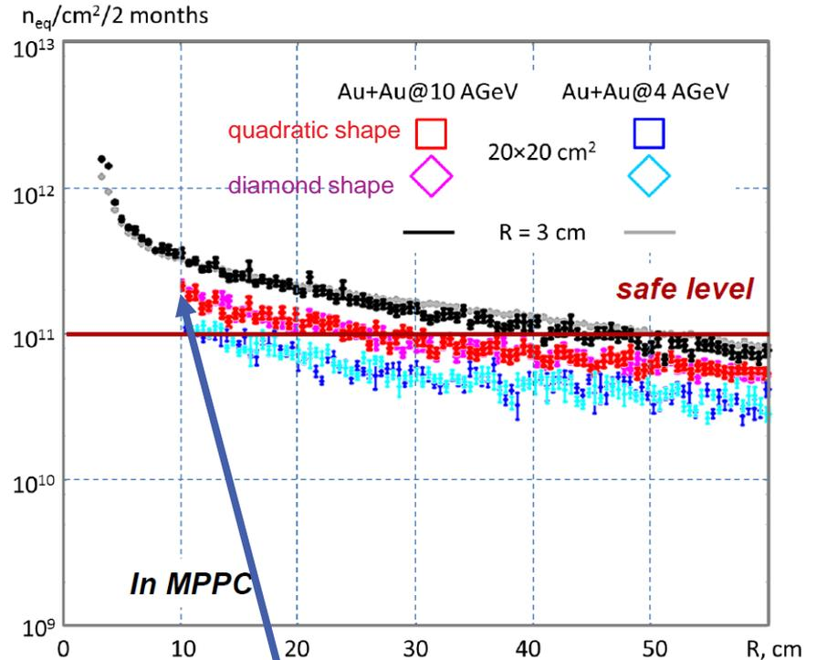
up to  $2 \times 10^{11}$  neutrons<sub>eq</sub>/cm<sup>2</sup> for SiPMs located 10 cm close to the beam center
