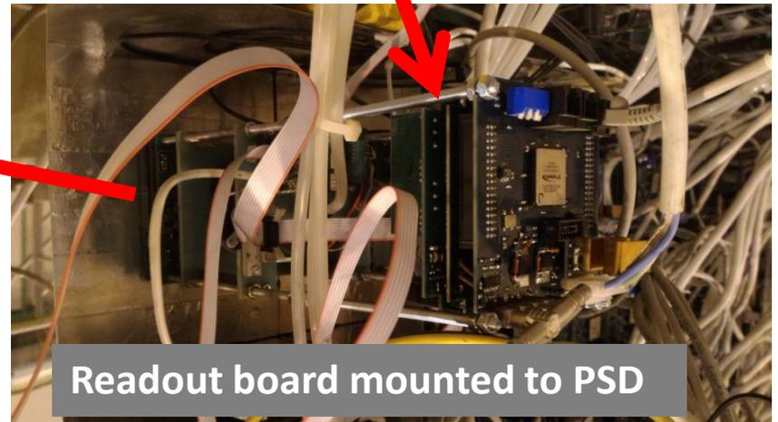
Readout board mounted to PSD
