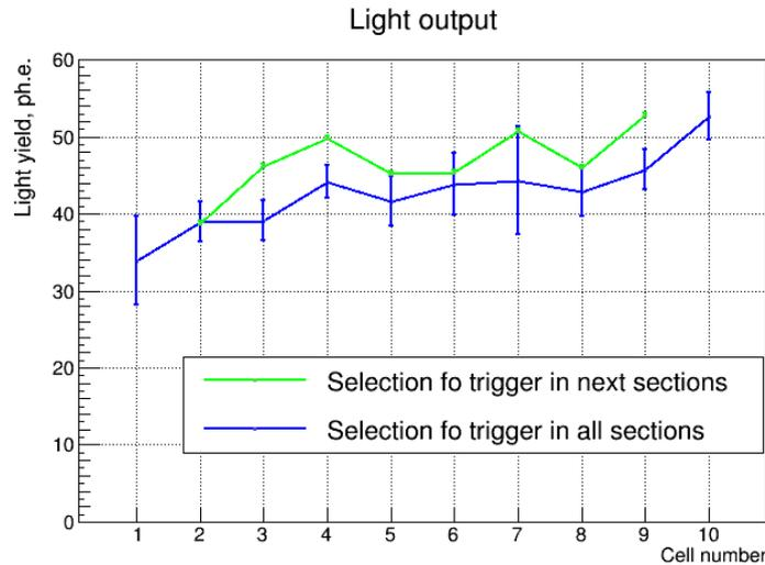
Light yield of each of 10 individual sections in module was measured by cosmic muons
