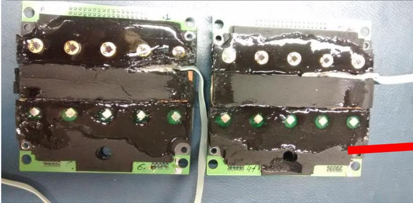
PSD readout board assembled
