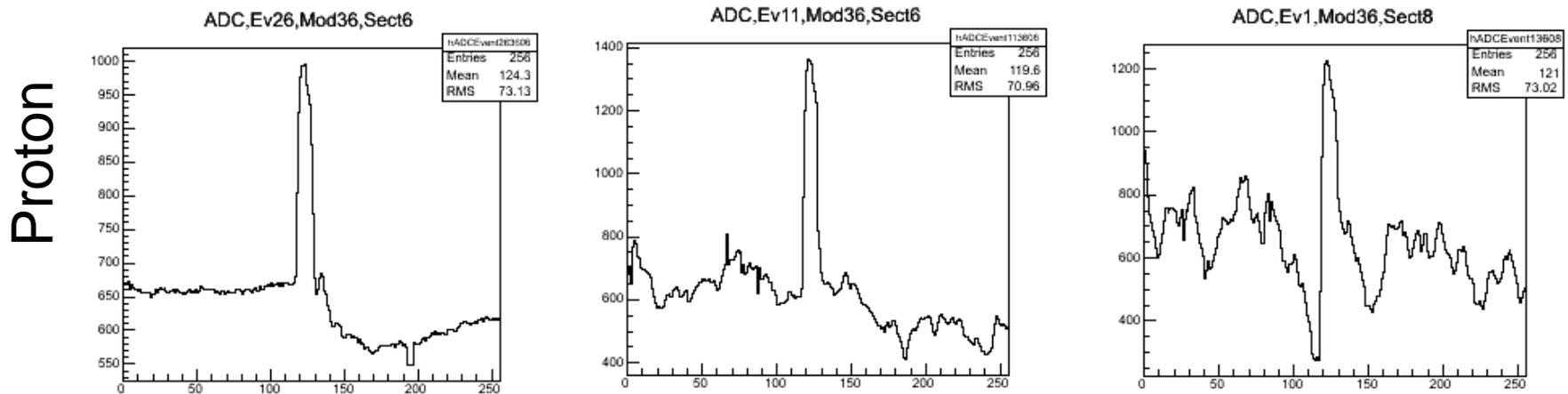
With the noise increased at 10-30 times SiPM cannot detect MIPs (~10-15 photons)!
