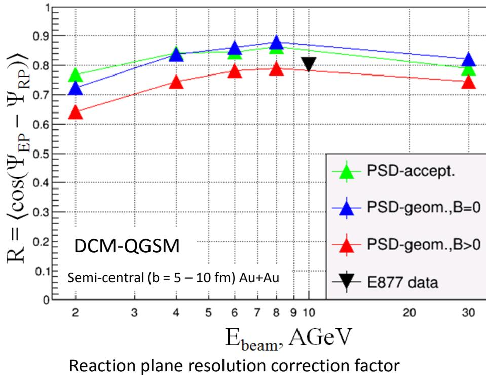
**PSD-accept.:** Reconstruction by MC-tracks with PSD acceptance ( $\vartheta$ -angle)
