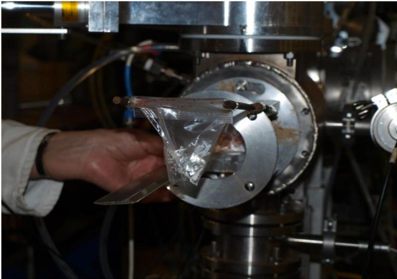
“White” neutron beam by Be(p) thick target
