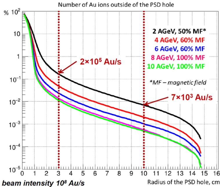
up to 30 times less ions hitting the calorimeter
