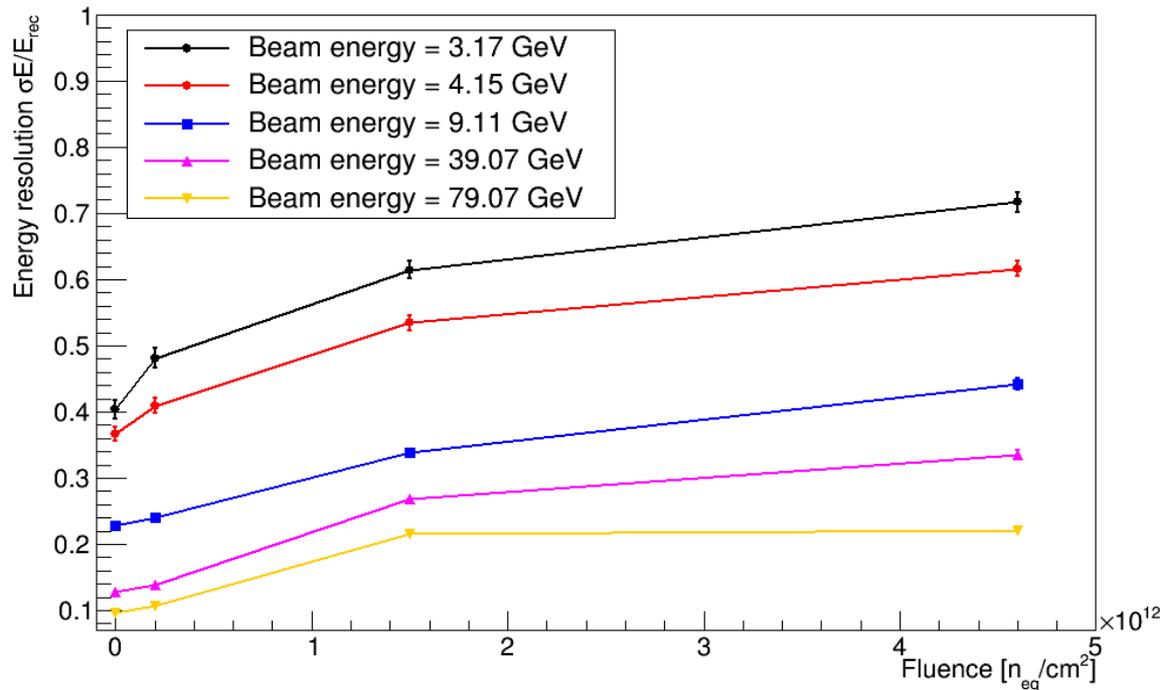
Single module energy resolution versus neutron fluence
