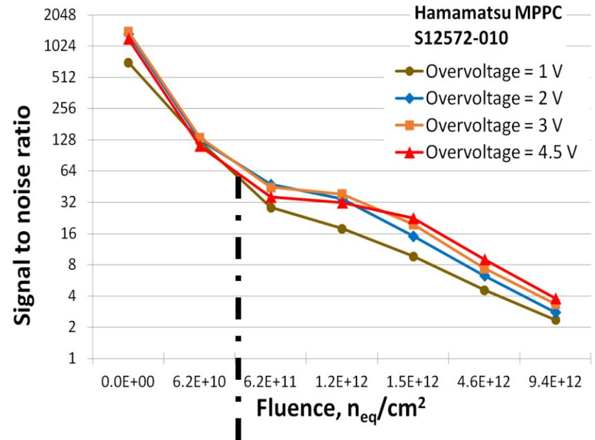
$$\text{Signal to noise ratio} = \text{Integral}_{\text{Signal}} / \sigma_{\text{Noise}}$$
