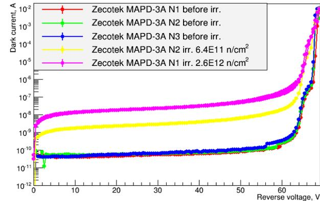
$$V_{\text{break}} = 65 \pm 0.2V$$
