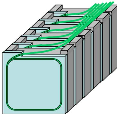
Light from each consecutive 6 layers is collected together via WLS-fibers and read-out by a single Hamamatsu Multi-Pixel Photon Counter (MPPC)
