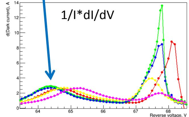
$$\Delta V_{\text{break}} (6.4e11 \text{ n/cm}^2) \sim 0.4V$$
