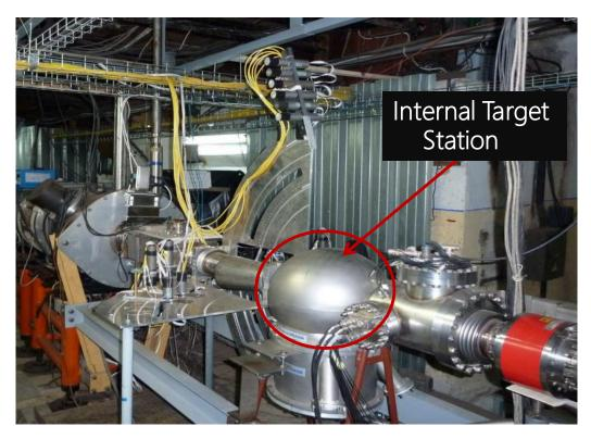
Internal Target Station is very well suited for the measurements of the deuteron- induced reactions observables at large scattering angles
