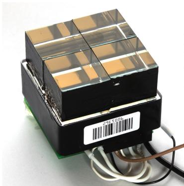
The **MCP-PMT XP85012** with 64 anode pads is transformed into the 4-channels detector by merging 16 pads ( $4 \times 4$ ) of each cell into a single channel
