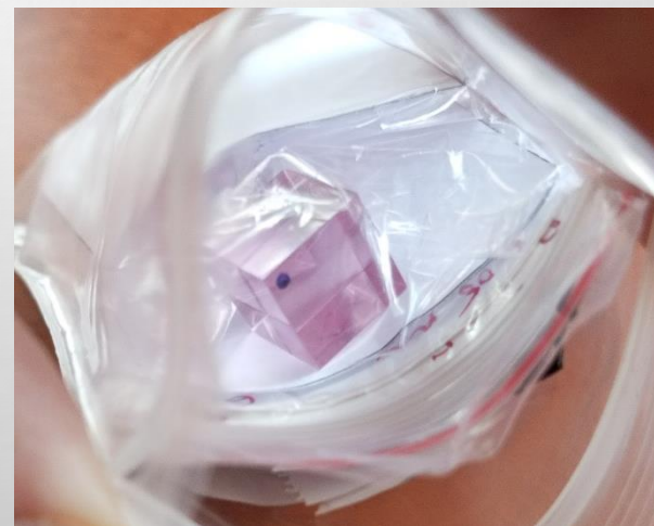
Color centers formation in the BaF 2 after 100 kGy absorbed dose.
