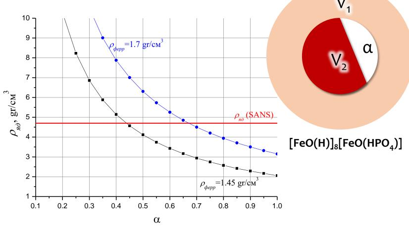
$$\rho_{core} = \frac{1}{\alpha} \left( \rho_{ferr} \left( 1 + \frac{V_1}{V_2} \right) - \rho_{apof} \frac{V_1}{V_2} \right) = \rho_{ferr} \left( 1 + \frac{R_1^3}{R_2^3} \right) - \rho_{apof} \frac{R_1^3}{R_2^3} = \mathbf{4.7} \ \mathbf{g/cm^3}$$
