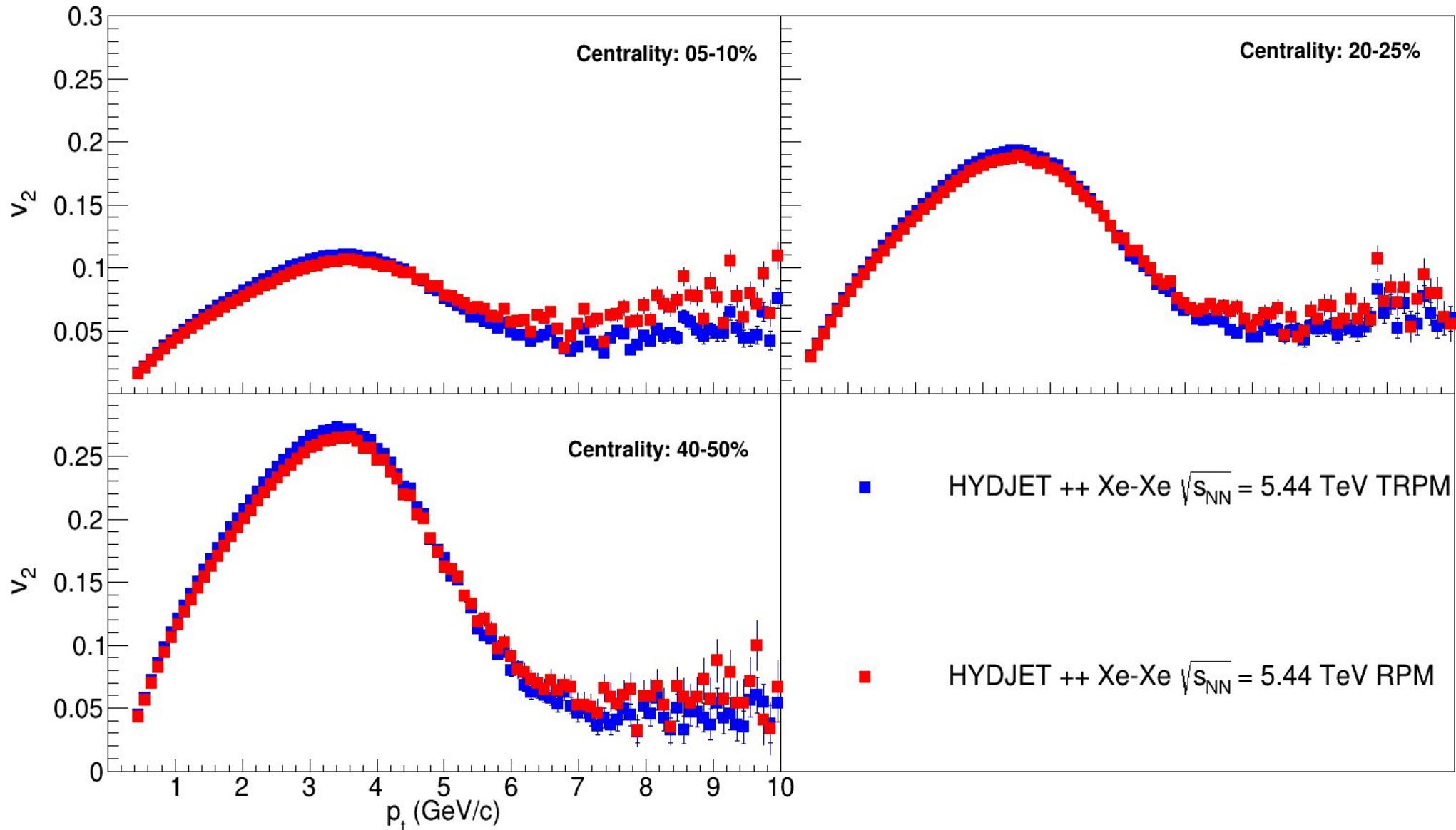
The results for the flows were obtained in the HYDJET++ generator (statistics approx. 1 million. events for each centrality true and calculated).
