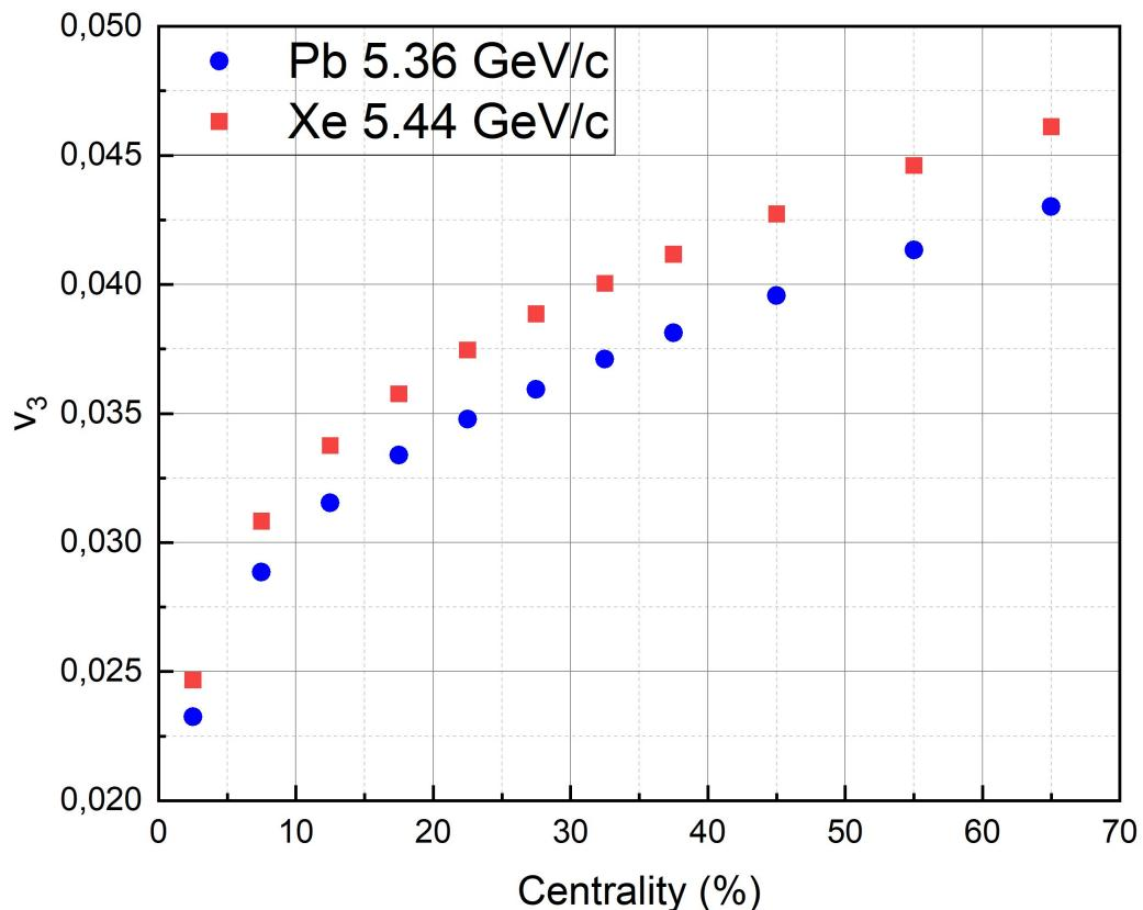
The results for the flows were obtained in the HYDJET++ generator relative to the true plane of the reaction (statistics approx. 1 million. events for each centrality).
